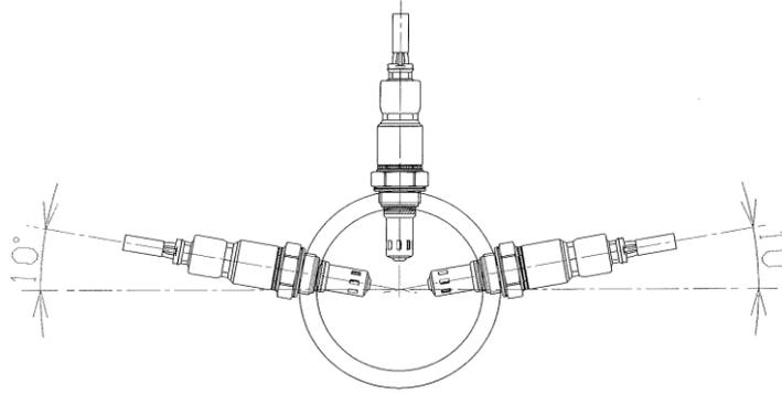
After welding the sensor boss to the exhaust, run an M18 x 1.5mm tap or thread cleaner (KD Tool P/N 730 or equivalent) through the boss to remove any thread-distortion. If this is not done, the sensor's threads may be damaged during installation or removal. Apply a small amount of anti-seize compound to the threads and tighten the sensor to 45~55N·m.(Previously stated as 1/3~1/2 turn)
