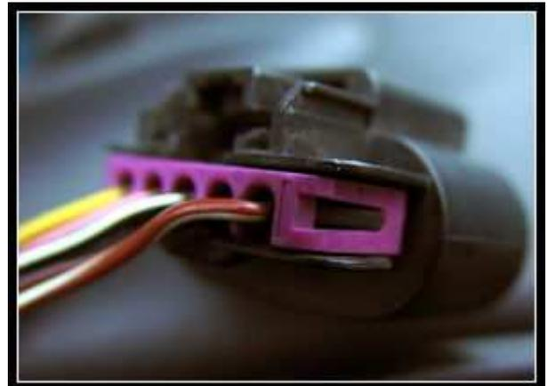
2. Starting with the rear retainer, lift the end of the locking tab up with a small screw driver and prise the retainer back, away from the plug. Do this on both sides to free the retainer.
