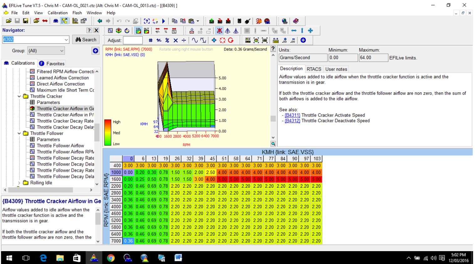
I also found that if my thermo fans would kick in the PCM wasn't compensating enough air, I changed the fans to .50 in the B4301 and B4302 tables. This fixed the issue with stalling with the fan on.
