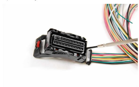
Leveraging the other end to the cable side out. The separator needs a light push upward to unclip it at each end.
