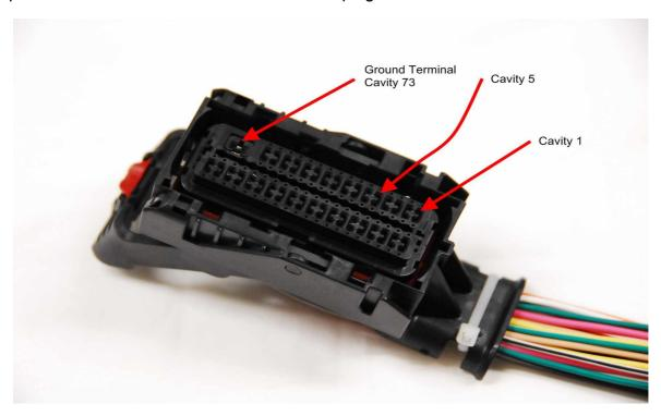
A small screwdriver is used to break the black moulded in plug loose. Push on the edge of the plug alongside the cavity wall for best leverage. It should break loose without too much pressure if you push in the right place.
