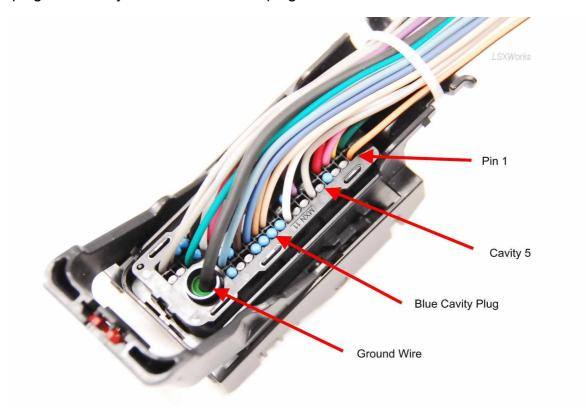
Flip side of connector - terminal side where it plugs in to ECM socket.
