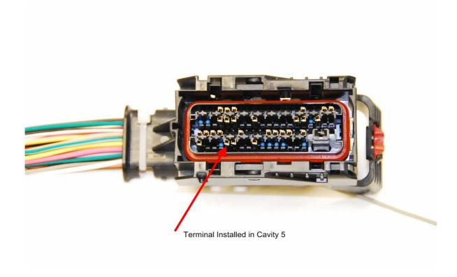
Connector with terminal separator re-installed. Only goes one way, with different sized tongues on each end, and the ground terminal.
