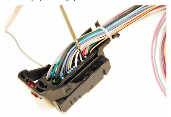
If your connector has the moulded in black plugs, they need to be removed from the terminal area underneath the terminal separator. Use a small screwdriver at each end of the separator to leverage it out. Cable end:
