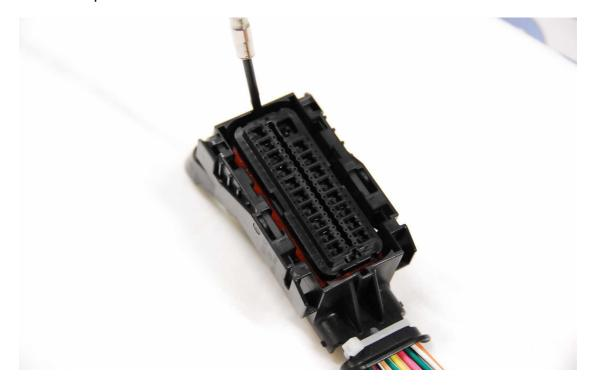
Look into cavity 5 for the moulded in plug and remove it with a small tool. Though some connectors may have no plugs, and open seals, this is unlikely.
