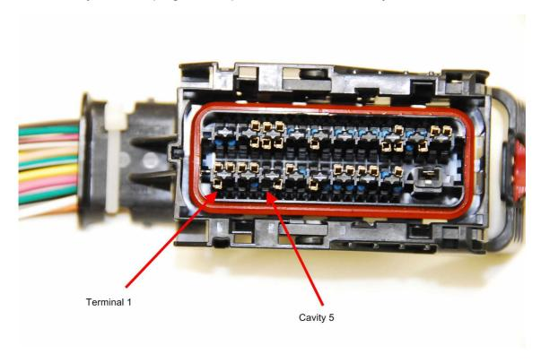
Terminal on the way in to the right cavity. Make sure it is oriented the right way around. There is an open section in the terminal which needs to engage a locking tang once pushed in.
