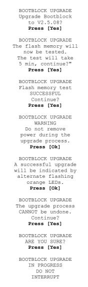
The upgrade process will take about 5 seconds to complete, then the screen backlight will be turned off (the text will be dark but just visible) **and the two orange LEDs will flash alternately to indicate dead-poll mode**. Dead-poll mode means that FlashScan is waiting to be programmed with new firmware. See "How to program new firmware into FlashScan" below.
