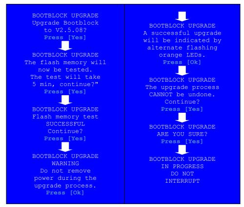
The upgrade process will only take about **5** seconds to complete, then the screen backlight will be turned off. The final message: BOOTBLOCK UPGRADE IN PROGRESS DO NOT INTERRUPT will still be visible. Once the backlight has been turned off that message no longer applies.
