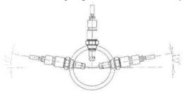
After welding the sensor boss to the exhaust, run an M18 x 1,5mm tap or thread cleaner (KD Tool P/N 730 or equivalent) through the boss to remove any thread-distortion. If this is not done, the sensor's threads may be damaged during installation or removal. Apply a small amount of anti-seize compound to the threads and tighten the sensor to 45~55N·m. (Previously stated as 1/3~1/2 turn)
