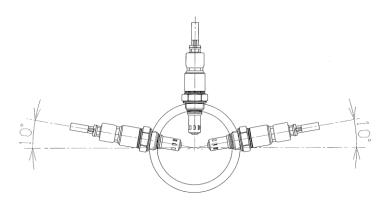
After welding the sensor boss to the exhaust, run an M18 x 1.5mm tap or thread cleaner (KD Tool P/N 730 or equivalent) through the boss to remove any thread-distortion. If this is not done, the sensor's threads may be damaged during installation or removal. Apply a small amount of anti-seize compound to the threads and tighten the sensor to 45~55N·m.(Previously stated as  $1/3\sim1/2$  turn)
